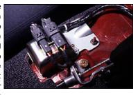
voltage decreases below 2.5 on right turns and increases above 2.5 volts on left turns.
