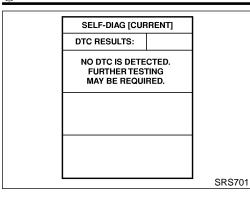
If no malfunction is detected on "SELF-DIAG [CURRENT]" but malfunction is indicated by the "AIR BAG" warning lamp, go to DIAG-NOSTIC PROCEDURE 4, page RS-33 to diagnose the following situations:
