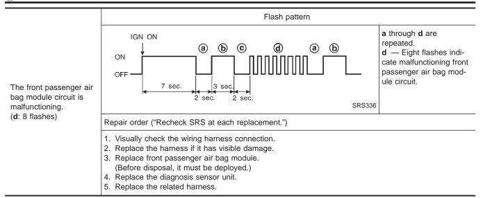
\* Follow the procedures in numerical order when repairing malfunctioning parts. Confirm whether malfunction is eliminated using the air bag warning lamp or CONSULT-II each time repair is finished. If malfunction is still observed, proceed to the next step. When malfunction is eliminated, further repair work is not required.
