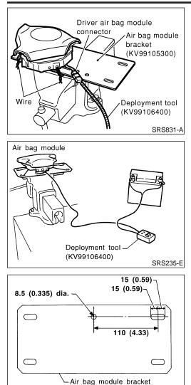
3. Connect deployment tool (SST: KV99106400) to air bag module connector.
