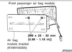
3. Match the two holes in air bag module bracket (held in vise) and passenger air bag module and fix them with two bolts [M8  $\times$  25 - 30 mm (0.98 - 1.18 in)].
